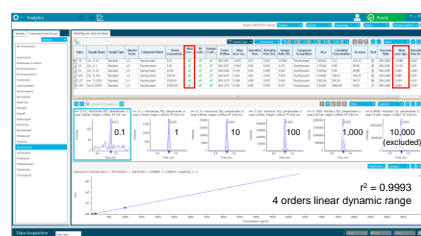
Figure 2. Linearity and mass accuracy for Paclobutrazol (0.1 to 10,000 ng/mL), linearity was achieved over 4 orders of magnitude, mass accuracy of less than 1 ppm was maintained even above the upper limit of quantitation ULOQ
